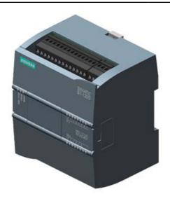
SIMATIC S7-1200, CPU 1212C, COMPACT CPU, DC/DC/RLY, ONBOARD I/O: 8 DI 24V DC; 6 DO RELAY 2A; 2 AI 0 - 10V DC, POWER SUPPLY: DC 20.4 - 28.8 V DC, PROGRAM/DATA MEMORY: 75 KB
